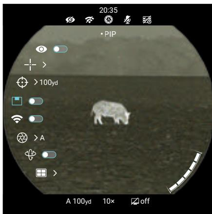
**NOTE:** If PIP is turned on, rotating the **Control Turret** will adjust the digital zoom level for the PIP image.
