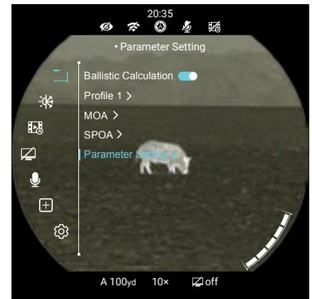
4. Rotate the **Control Turret** to move through the parameter options.
