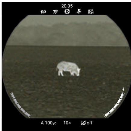
The fill level of the active battery status indicator indicates the current battery charge level. The battery charging ⚡ icon appears above the built-in battery status indicator when the ACE Series is connected to an external power source. See the table below.
