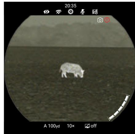
**NOTE:** A red warning icon (⚠️) appears next to the camera icon in the upper-left corner of the screen when insufficient memory storage is available. Transfer video and image files to other storage media to free up space on the memory card.
