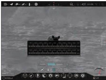
9. Use the **Rotary Encoder** to customize the shooting table. Rotate to move through the range inputs in the table, short press to add data to a table cell, and long press to save the data point and exit the cell.
